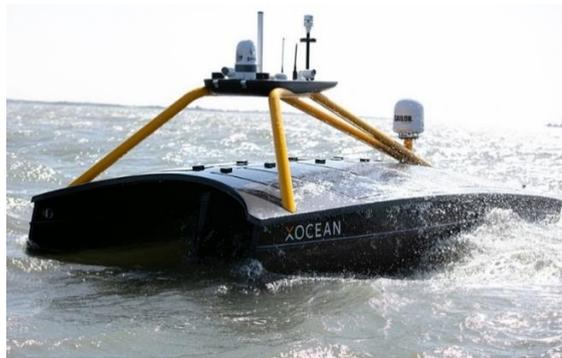
The USV sends real time images and situational awareness data over satellite to a team of operators keeping watch and controlling the vessel remotely 24/7.
