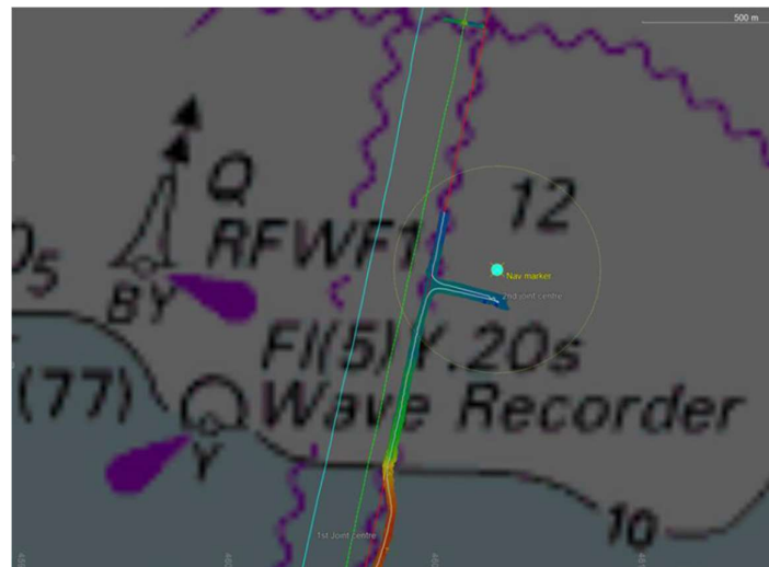
Figure 1 Cable repair loop and marker buoy overview
