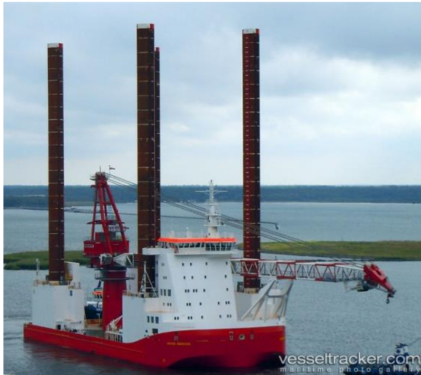
Jack up vessel WIND SERVER
