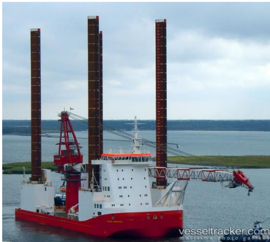
Jack up vessel WIND SERVER
