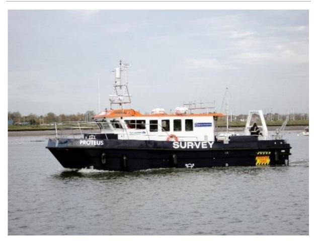
MV Proteus is a 14m x 5m GRP catamaran hull design coastal survey vessel .The lower sections of the hull and dark blue and the upper sections and wheelhouse are white, with 'SURVEY' lettering in white
