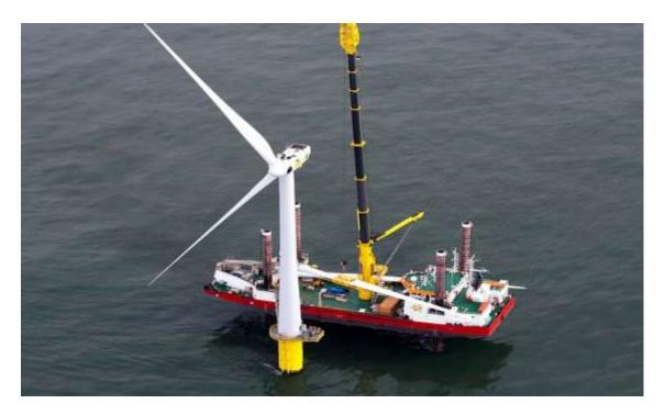
The Wind is a Jack-Up platform(Wind Farm Installation Vessel) measuring 55 metres in length and has a 4.3 metre draft, coloured Red and white. When jacked up the Wind will be marked and displaying lights and day symbols in accordance with an Offshore Structure.
