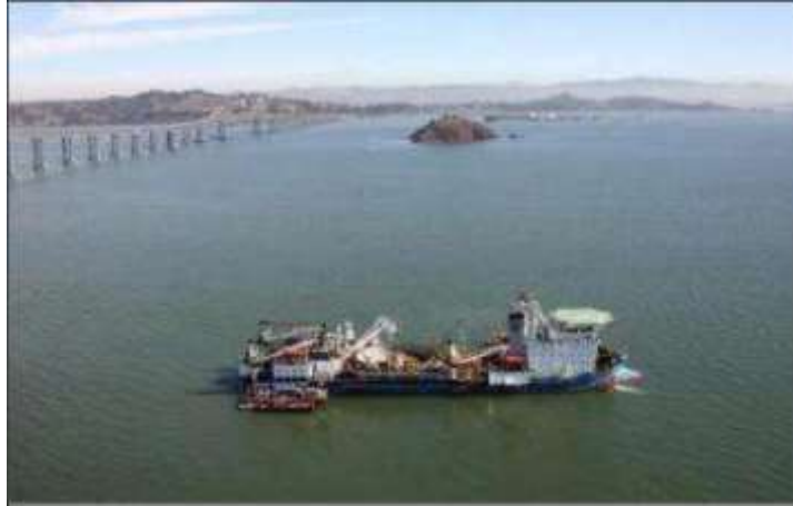
Figure 1 Cable Laying vessel - Giulio Verne
