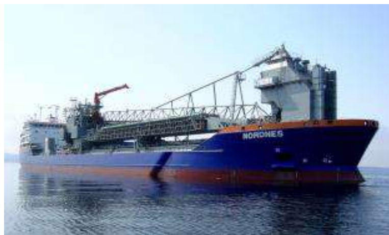
Rock Placement vessel - Nordnes
