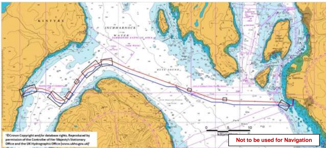
North and South Cable Routes with Areas Marked (black boxes) for Rock Placement
