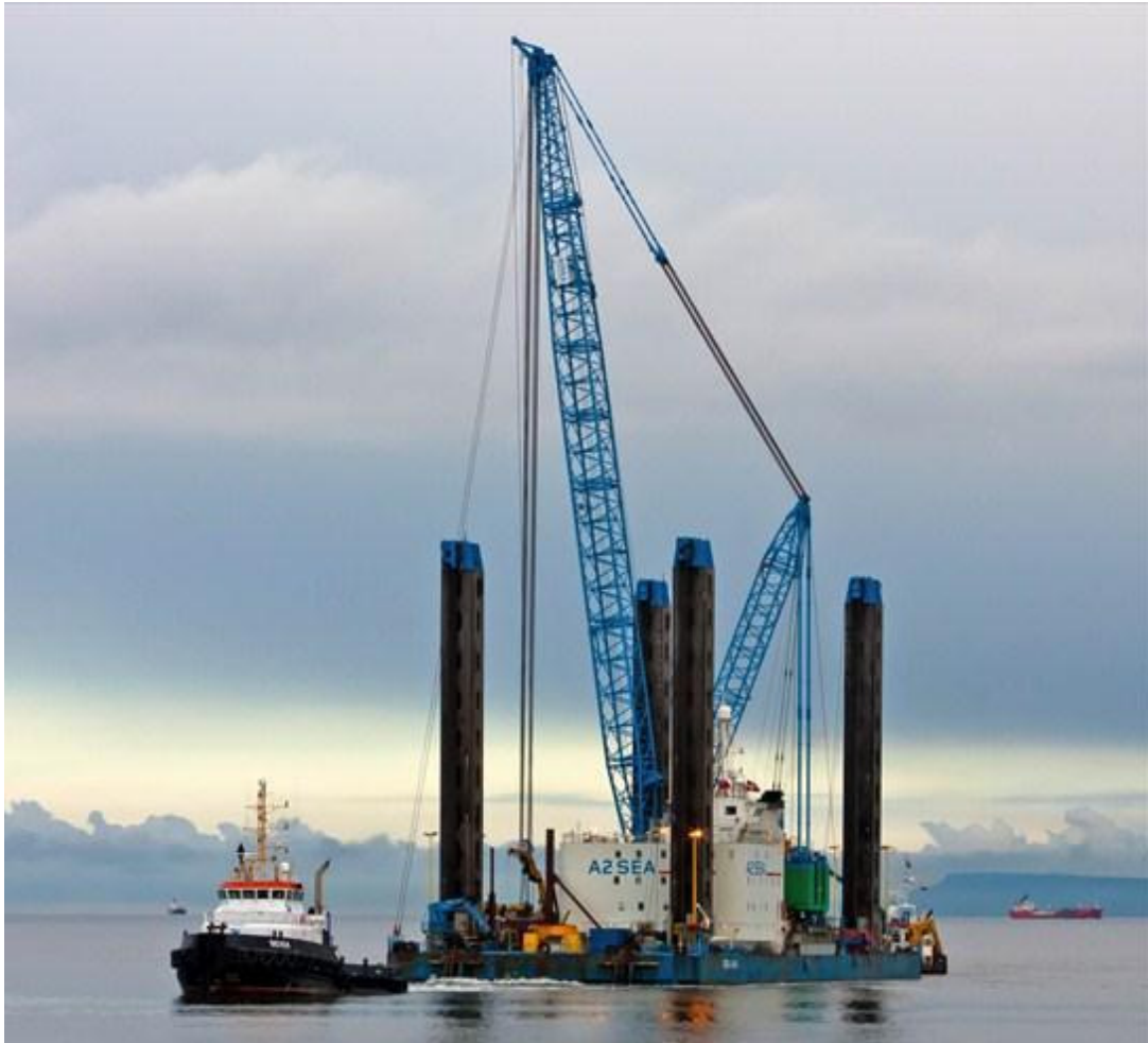
A2Sea Sea Jack[self elevating Turbine installation vessel]
