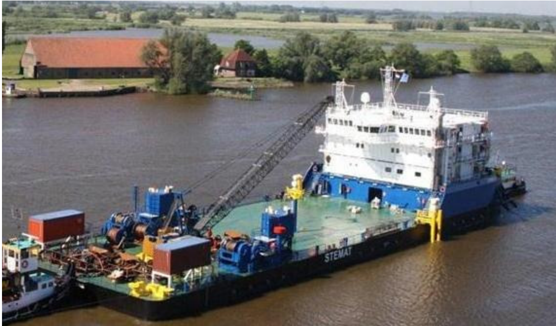
Stemat 89 Cable Jointing Vessel[Multi purpose barge]
