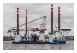
RWE's new wind farm installation vessel (left), has successfully completed jack-up trails in Liverpool Bay. The Friedrich Ernestine, has been built and designed by RWE Innogy and will carry out installation activities on the project. At 100 metres long and 40 metres wide, the vessel is one of the largest of its kind in the world
