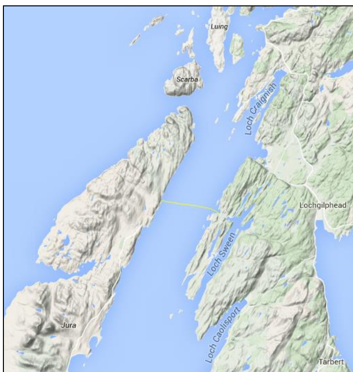
Route of the Mainland-Isle of Jura Electricity Cable (Source: KIS-ORCA).
